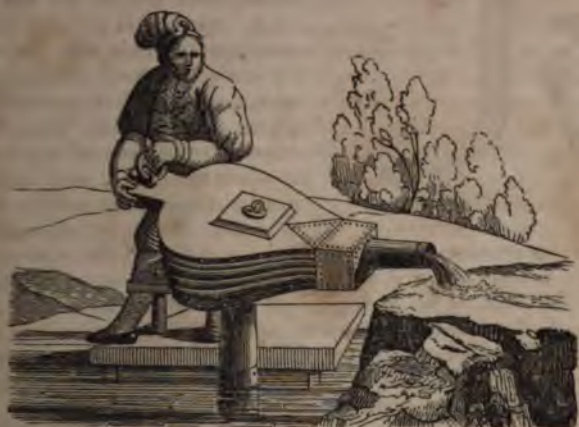
No. 82. German Atmospheric Bellows Pump. A. D. 1511.
